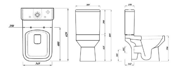
**Special notes**Pan fixes to floor using side fixing bracket supplied with pan.
