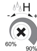
The humidity level is adjusted by turning the potentiometer clockwise to increase and anti-clockwise to decrease. To set the maximum humidity level the potentiometer has to set at the max position (90%).
